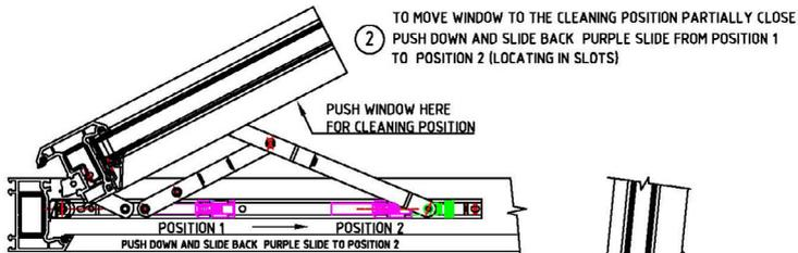
③ USING THE HANDLE - OPEN THE WINDOW TO THE CLEANING POSITION
